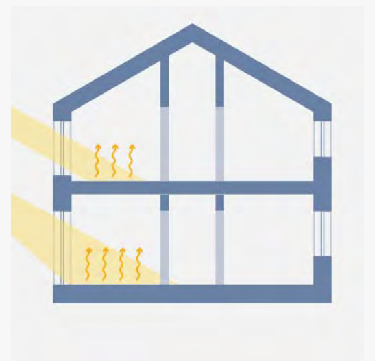
Fig: Passive Heating Systems
